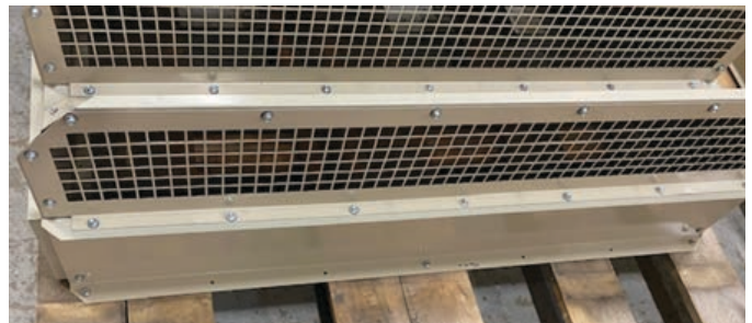
Figure 78: Side panel of hood (one on both sides) needed to be removed to secure hood
