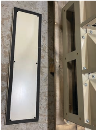
Figure 80: Side flange to be secured once side panel is removed
