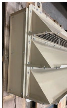
Figure 78: Side panel of hood (one on both sides) needed to be removed to secure hood
