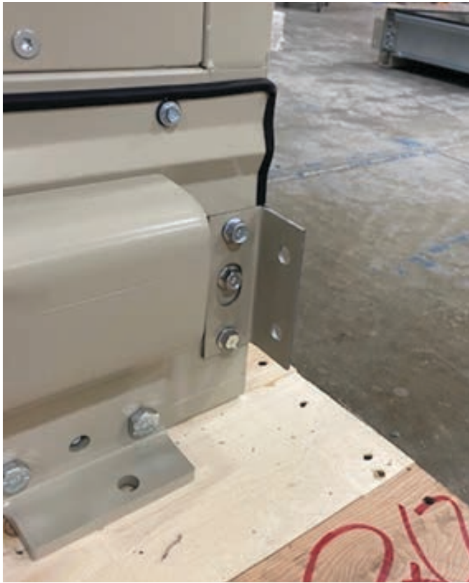
Figure 84: Lifting lugs located on base rail
